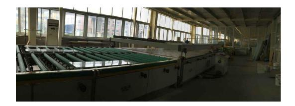
Next, it is fired within a tempering furnace to create a permanent coating. The glass is always either heat strengthened or fully tempered to prevent glass breakage due to thermal stresses under sunlit applications.
